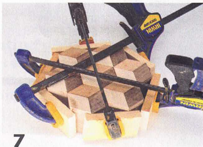
7 From a separate example, 2"-tall cells are glued into a seven-cell core.
