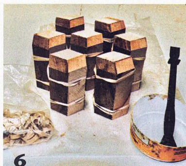
6 Segments are glued up into seven 4"-tall cells, with gluing pressure provided by rubber bands. After the glue dries, the cells are sanded lightly.
